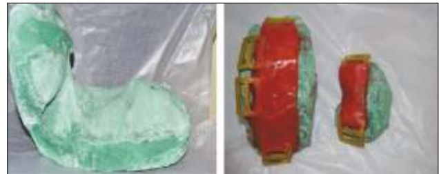
Fig.04 : Stone cast and wax patterns
