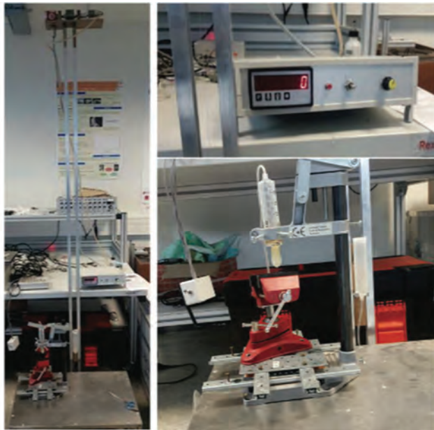
Fig. 2 Global view of the calibration device (left); latex finger and vice holding the denture (right bottom); and electric motor display showing the height of the water (right top).
