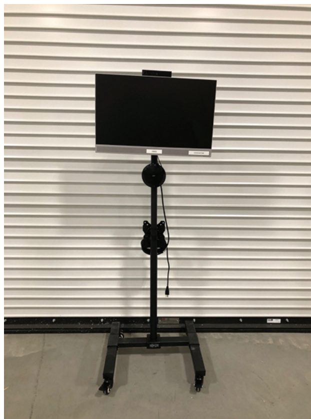
Fig. 1 Example cart built for medical/surgical units, all-in-one computer with built-in fixed camera.
