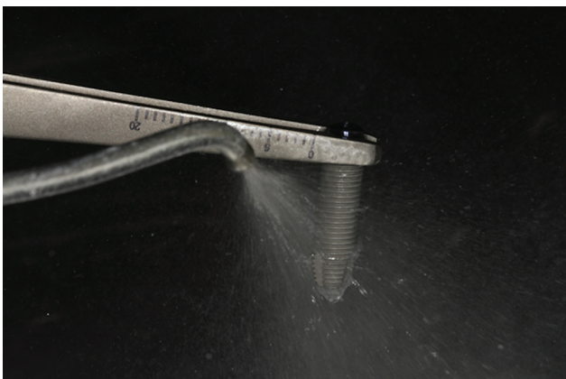
Fig. 2 Dental implant receiving air-powder abrasive system with sodium bicarbonate for 1 minute.
