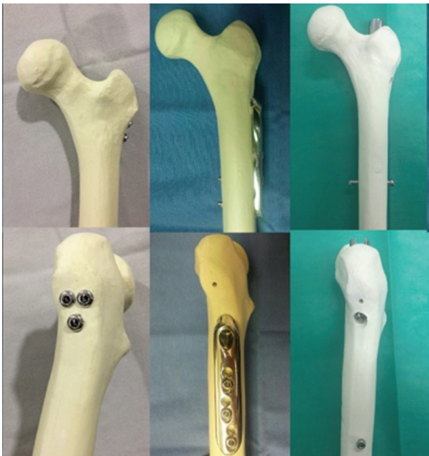
Fig. 2 Cannulated screw (CSG), dynamic hip screw (DHSG) and proximal femoral nail (PFNG) group samples after implant placement.
