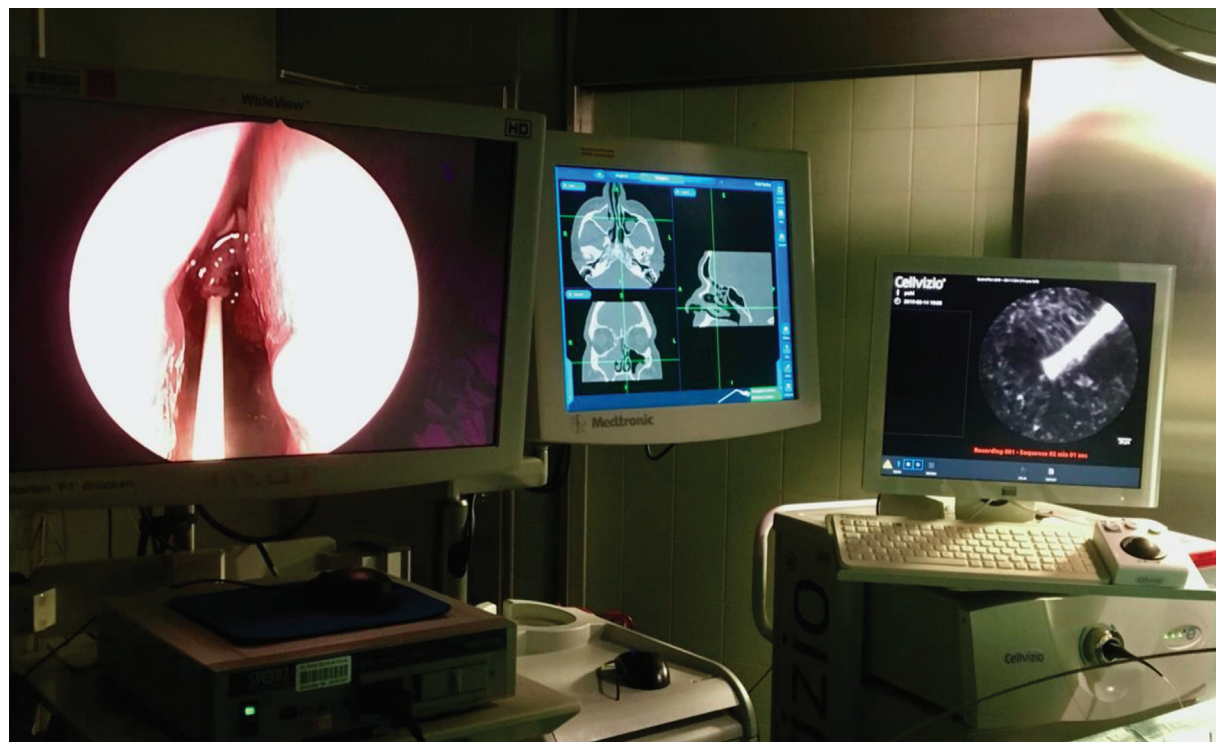
Fig. 1 Intraoperative setting from left to right: AIDA system for functional endoscopic sinus surgery, computed navigation (Medtronic) and confocal laser endomicroscopy (Cellvizio).
