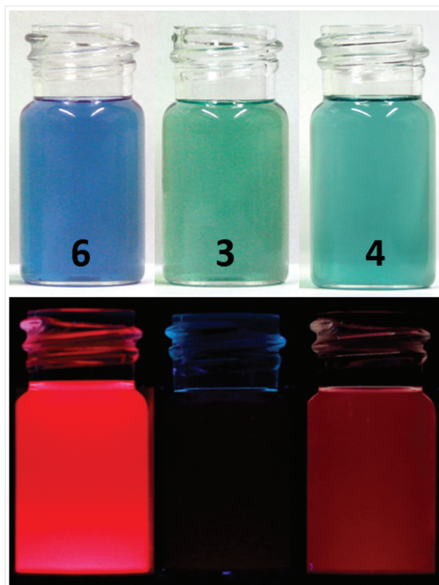
Figure 2 Photographs of monomer 6 (left), dimers 3 (middle) and 4 (right) under daylight (top) and UV light with excitation at 365 nm (bottom) in n -hexane.
