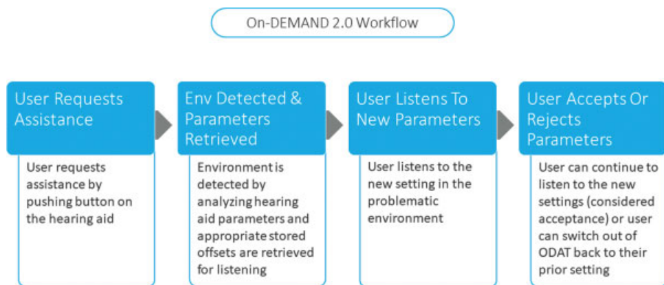
Figure 3 Workflow for on-demand adaptive tuning (ODAT), known as “Edge Mode.”
