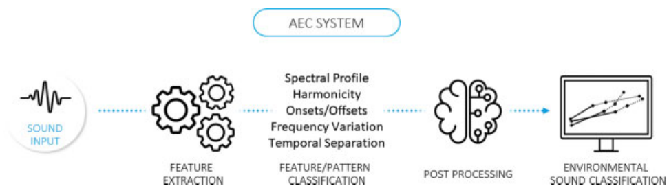
Figure 2 Block diagram of an acoustic environmental classification (AEC) system incorporating feature extraction, feature/pattern classification, post-processing, and environmental sound classification.
