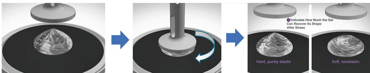
**Fig. 1** Schematic representation of a rheometer in oscillation mode. The gel is placed between two plates of defined geometry to assess elasticity (solid behavior) quantified by the elastic modulus, or  $G'$ , indicating how much the gel can recover its shape after shear stress. The same experiment also measures  $G''$ , the viscous modulus. From these measured parameters,  $G^*$  and  $\tan \delta$  ( $\delta$ ) can be calculated.<sup>11,17,20</sup>
