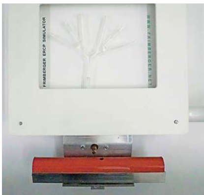
Fig. 2 B II/Roux-en-Y simulator. The sliding carriage, which is otherwise not visible, is pulled out for insertion of the papilla. The duodenum is mounted onto the carriage. In the window, the transparent bile duct is visible.
