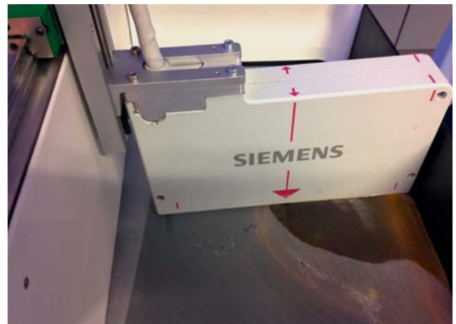
► Fig. 1 The ultrasound probe – taken from the ABVS ultrasound machine – moves over the compressed (elastic gauze) breast phantom.
