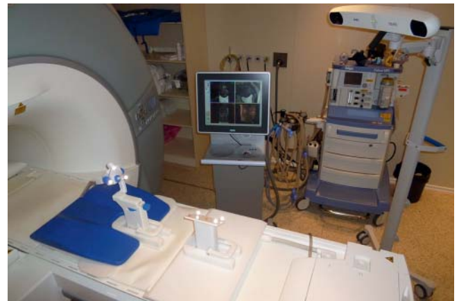
► Fig. 6 Navigation system for MR-guided biopsy of the prostate at a 3-T scanner. After registration of the biopsy device (Invivo, Schwerin, Germany) the navigation system (Localite, St. Augustin, Germany) reconstructs from the optically detected orientation of the biopsy device the corresponding MR slices and depicts them continuously on the in-room monitor.
