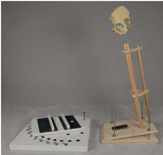
► Fig. 1 Rotatory platform (left) and rack for a test pelvis (right) to simulate pelvic tilt and rotation.
