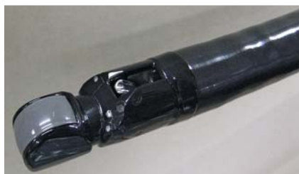
▶ Fig. 1 The new forward-oblique view convex-array echoendoscope, with 40° forward viewing direction.
