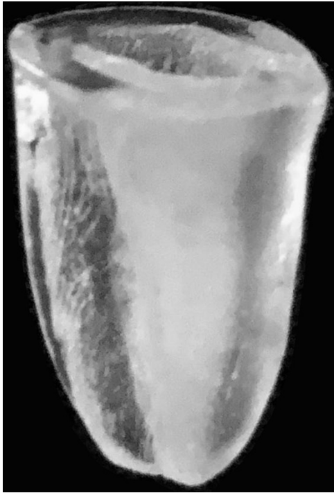
Fig. 1 Three-dimensional (3D) replicas printed on resin (VeroClear 810, Stratasys Ltda, Rehovot, Israel).
