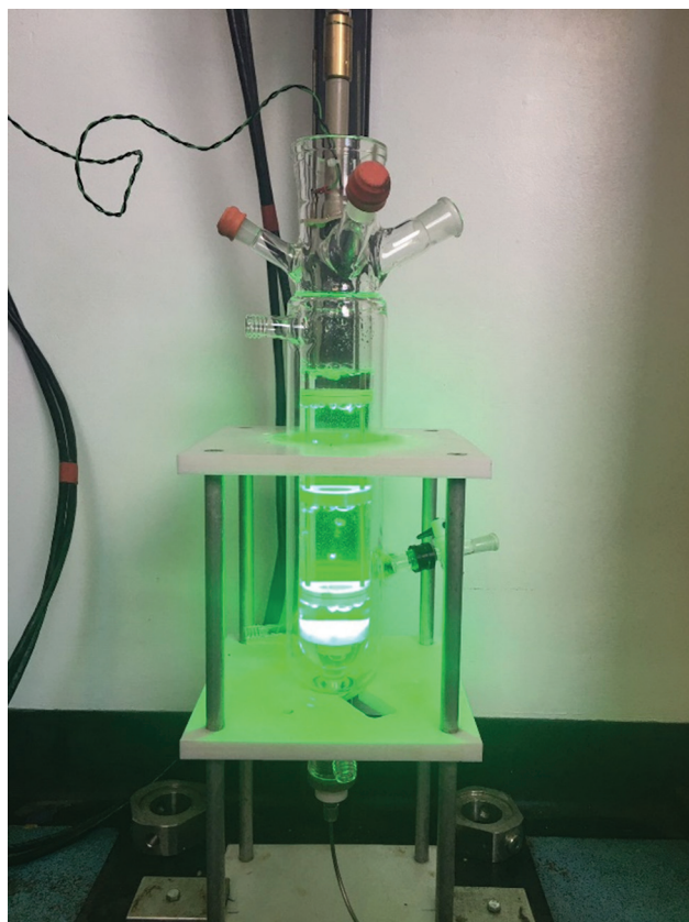
Fig. 3 The schematic of OBPR reactor and orifice baffles with LEDs. OBPR, oscillatory baffled photo reactor.
