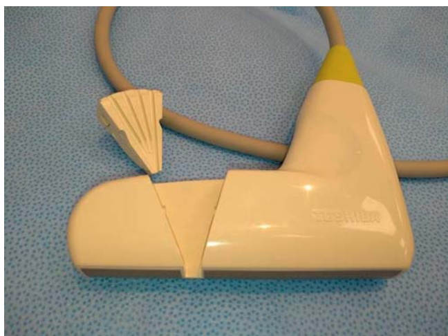
► Fig. 7 Ultrasound probe with puncture channel with removed needle guide. As a rule, these ultrasound probes and needle guides must be sterilized since the needle in the channel touches both parts.
