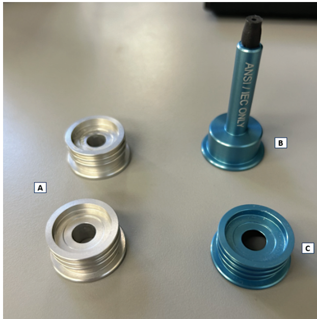
Figure 4 Couplers that are used to obtain the various measurements. (A) Silver (0.4 cc) couplers; (B) blue HA-2 (2 cc) coupler; (C) blue HA-1 (2 cc) coupler.
