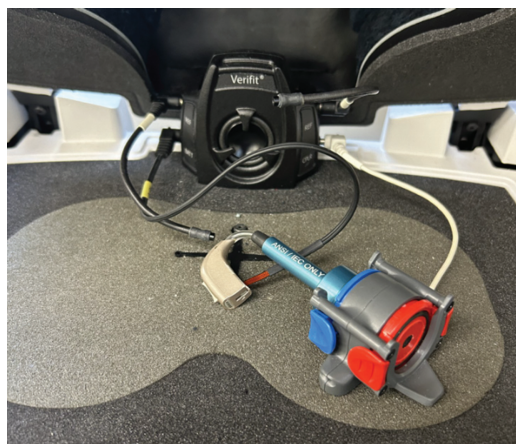
Figure 12 Connecting a hearing aid to the correct coupler with the battery pill in place.
