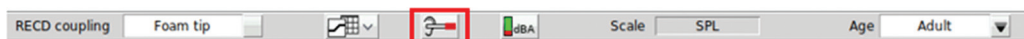
Figure 2 Probe guide button. Note that "adult" must be selected under the Age dropdown menu to use this feature. The feature was developed using data from a variety of adult ears, 5 which cannot be generalized to pediatric ears.
