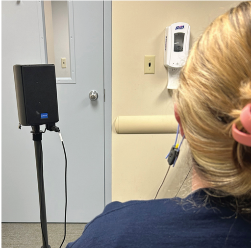
Figure 16 Setup for open-ear measurement of the normal hearing ear (probe microphone in left ear only, speaker at 45 degrees).
