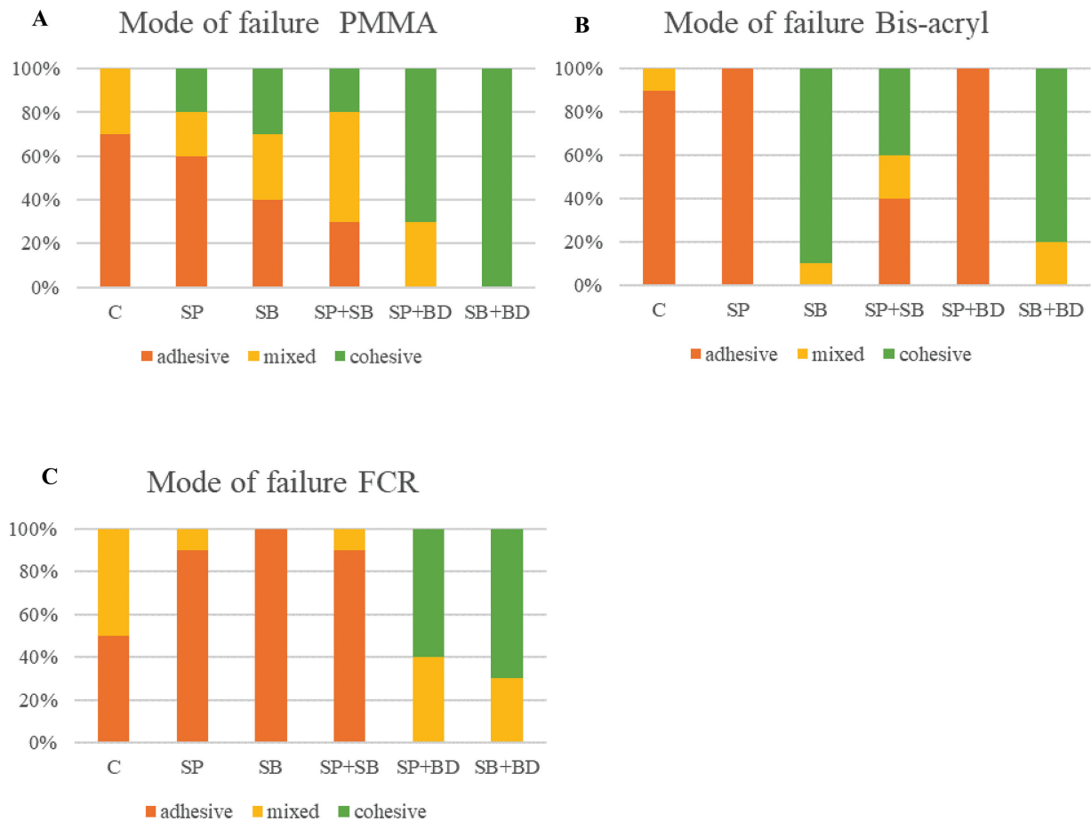
Fig. 4 Mode of failure in percentage for each material. (A) PMMA. (B) Bis-acryl. (C) FCR. C, control; BD, bonding; FCR, flowable composite resin; PMMA, polymethyl methacrylate; SB, sandblast; SP, silicon carbide paper.
