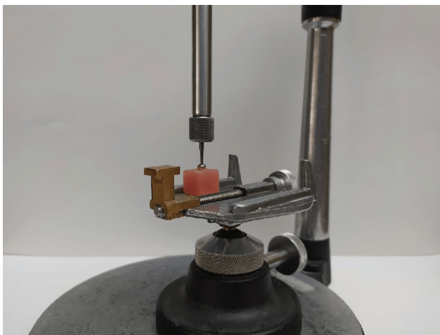
Fig. 1 Mounting the abutment in an acrylic resin block using a surveyor.
