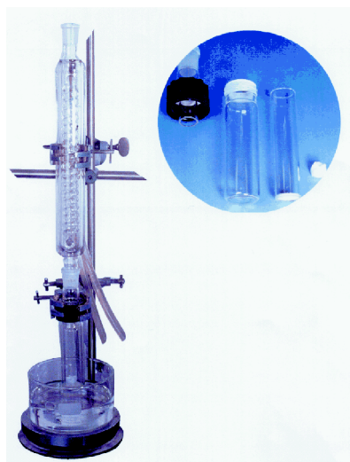
Figure 8. Inset: Reactor with glass frit, container, stirbar and connector. Main picture: Reactor in container and on top a reflux condenser.
