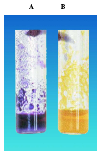
Figure 4. Bromophenol blue test with A) methylamine resin, and B) Wang resin.
