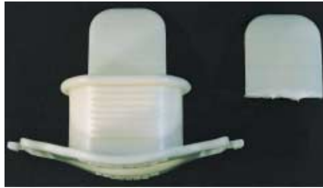
Figure 2 Comparison of the removed mouthpiece fragment with an intact mouthpiece
