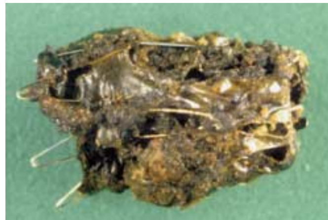
Figure 2 The exposed area of metallic stent with the conglomerated fragments of stone, and the distorted covered area of the stent with polytetrafluoroethylene material, after washing.
