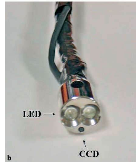
Figure 1 a The spectral characteristics of the new white light-emitting diode (LED) with the main peak of luminous intensity in the red range (600 nm). b Appearance of the prototype new white LED-illuminated endoscope (CCD, charge-coupled device).
