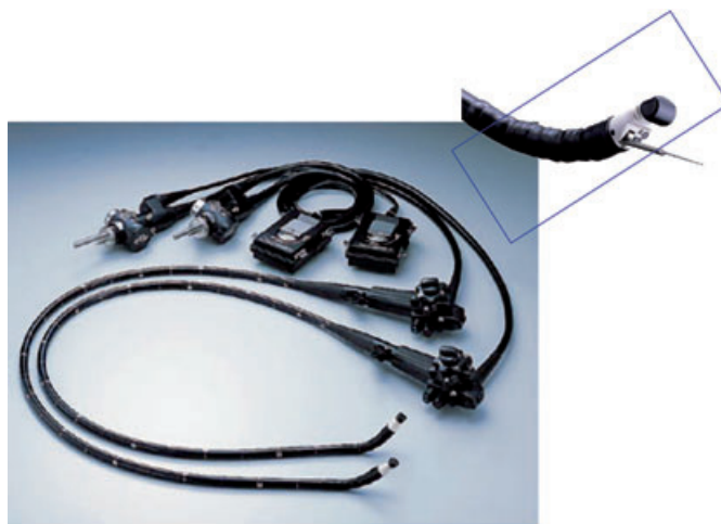
Fig. 1 Tipp of the linear array ultrasonic bronchoscope (BF-UC160F-OL8, Olympus Ltd., Tokyo Japan).
