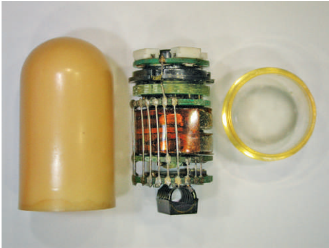
Fig. 4 The capsule disintegrated into three parts (the optical dome, the plastic body, and the capsule's internal components) after its removal from the ileum at autopsy.
