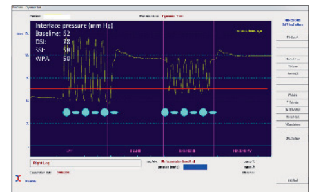
Fig. 4 Pressure curve of an inelastic bandage exerting a supine pressure of 60 mm Hg. Compression pressure increase by dorsiflexions, standing up and walking is very high: intermittent compression with high pressure peaks that overcome the intravenous pressure (represented by the red line) restoring a kind of valvular function.
