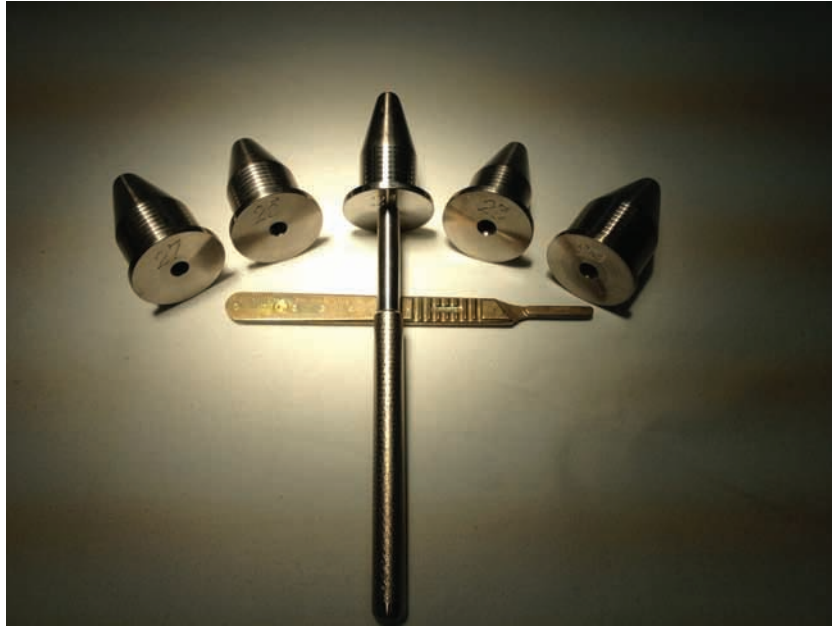
Figure 1. The new device, which has changeable cylinders with different diameters.
