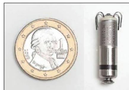
Fig. 4 The Medtronic Micra TPS leadless wireless pacemaker
