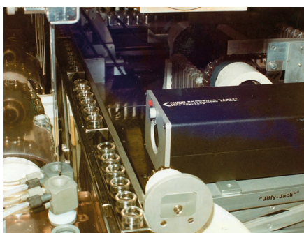
Fig. 16 AutoChemist could even be equipped with laser barcode readers for reading barcodes from every sample tube. Image from MetPath laboratory, New York, USA.
