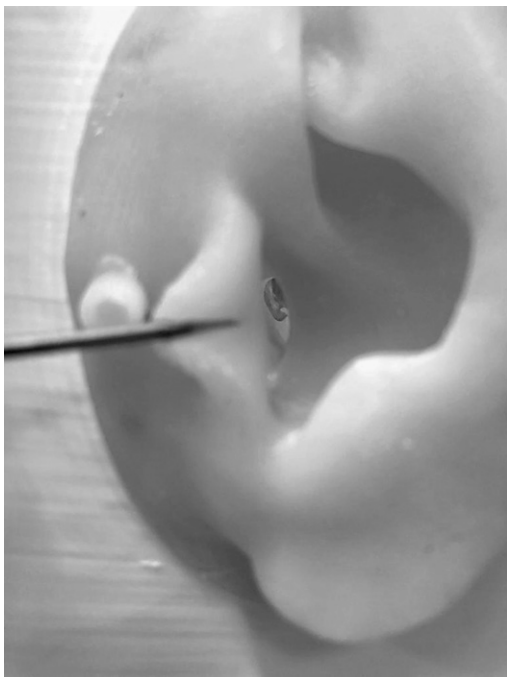
Figure 2. Image of the silicone ear model with the tragus moved aside showcasing the auricle, ear canal, and TM.
