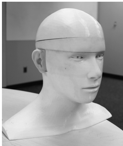
Figure 1. Image of the new probe-tube placement training simulator with a 3D-printed head and silicone ear model. The camera system is mounted inside the head to give the user real-time feedback on the placement of the probe inside the ear canal.
