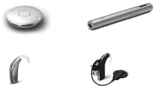
Fig. 2 Assistive technology used by the participants included Phonak Roger Select and Roger Pen microphones (top left and right) and Phonak Naida v90 SP/UP HAs with integrated Roger 18/19 receivers and N6 CIs with euroadapters and Roger X receivers (bottom left and right). (Photos courtesy of Phonak) (This figure appears in color in the online version of this article.)
