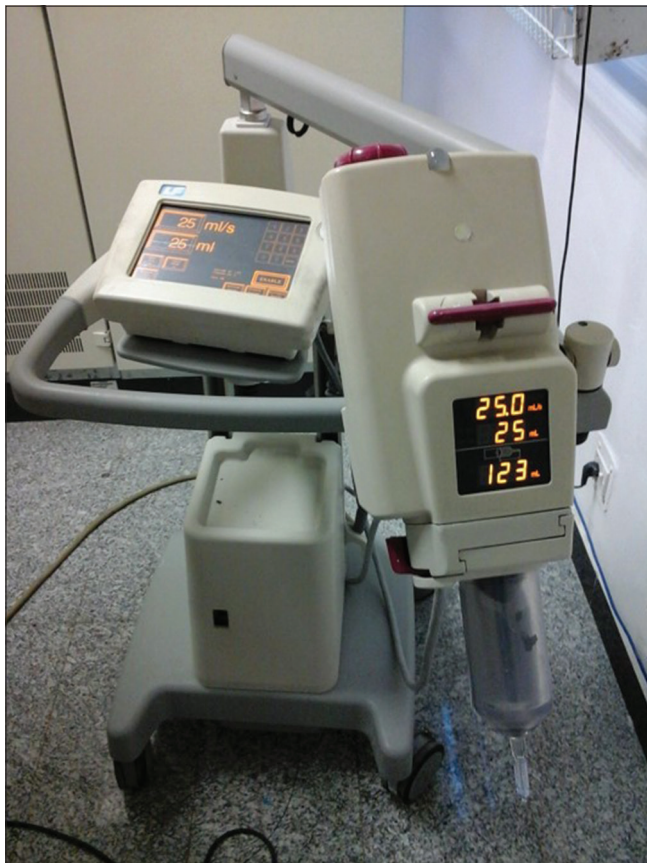
Figure 4 (A-C): Angiography / DSA Pressure Injectors (Liebel-Flarsheim). Few functional issues include (A) light, manoeuvrable and small footprint (B) protocols with variables of phase, volume, rate and delay (C) wide range of injection rates upto 45 ml/sec for aorta
