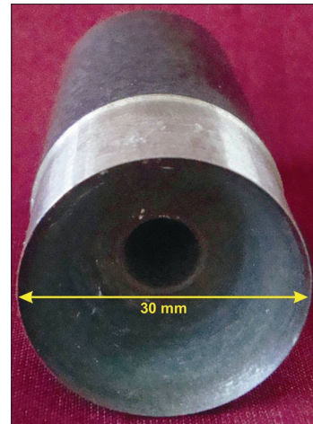
Figure 1: Die used for cutting of plastic strips
