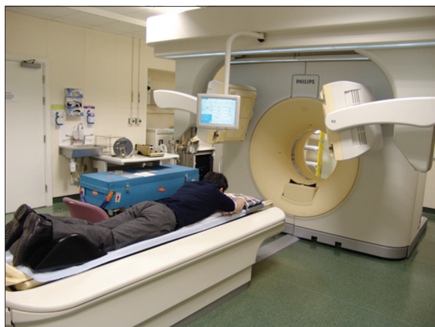
Figure 2: The dual-head gamma camera single photon emission computed tomography/computed tomography system – Philips Precedence 16
