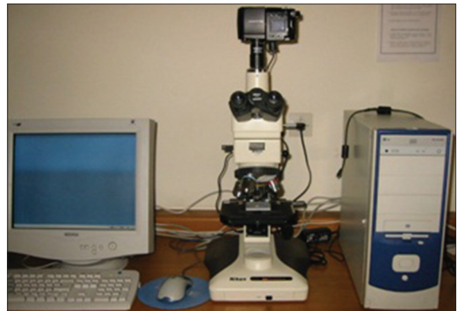
Figure 7: Measuring microscope (Nikon Optihot-100, Japan)
