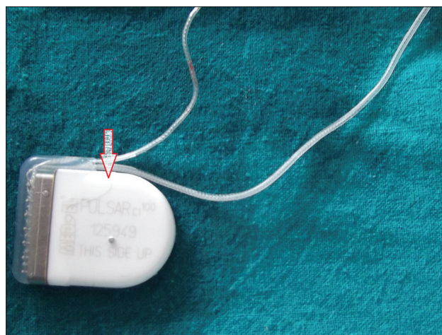
Figure 9: Fracture line on the receiver stimulator
