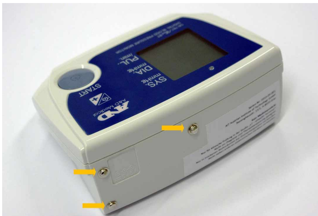
Fig. 1 Picture of modified digital blood pressure monitor UA-767 with three metallic dry electrodes (yellow arrows) to be touched with the fingertips of both hands (right hand: forefinger and middle finger, left hand: forefinger) or applied to the naked chest.
