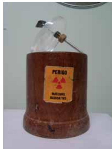
Figure 5. Strontium container plate (betatherapy).
